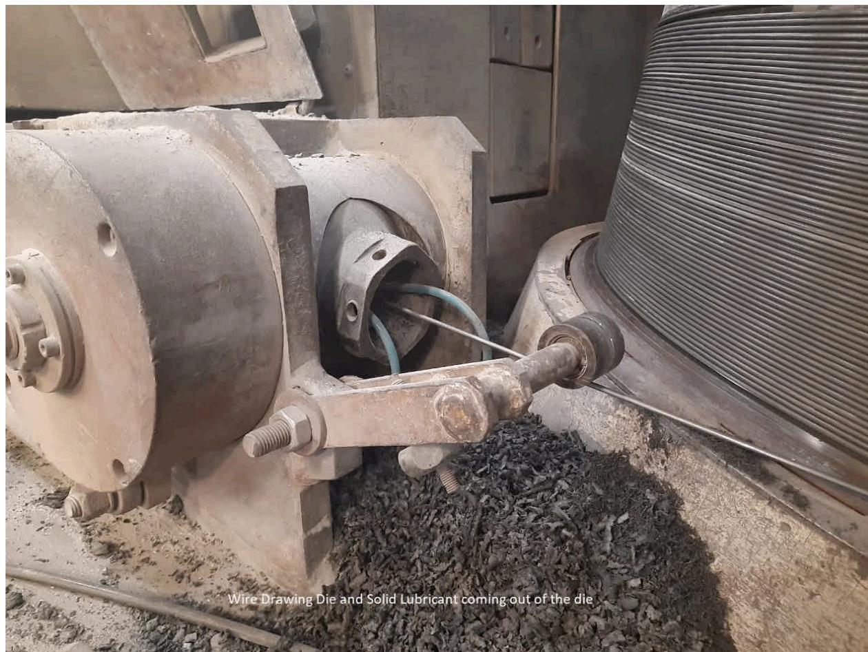
Wire drawing die with solid lubricant.
